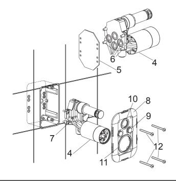
Remove the protection(5) on the valve kit(4). **NOTE**: Don't drop the o-rings(6).
