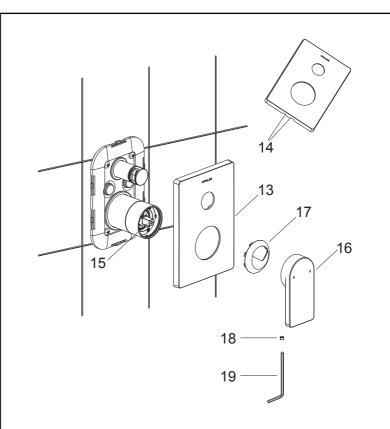
Slide the faceplate(13) onto the cover kit with slots(14) downwards. Push it against the wall. For ease of installation, push up the valve stem(15) for about 12° degrees.
