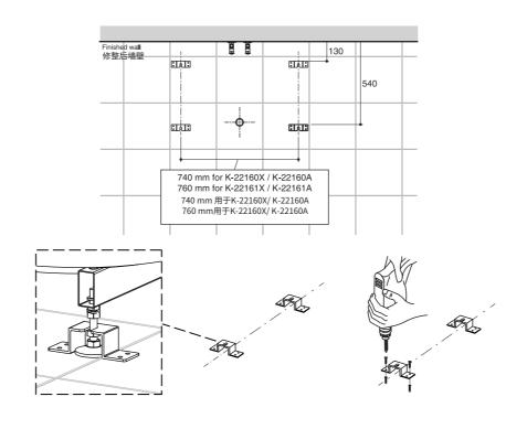
3. Carefully lift the bath into position. Ensure the bath is located right above the feet mounting clip.
