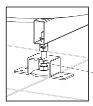
Adjust the nut to fasten the bath to the clip. 调整螺母,将浴缸紧固到安装夹上。
