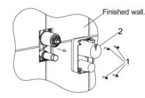
Apply a ring of plumbers putty around the back surface of the faceplate(4). Slide the faceplate on the valve(3). Push it against the wall. Remove any excess putty.
