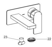
Ensure that all coupling nuts are tight. Ensure that the lever handle is in the off position. Turn on the main water supply and drain, and check for leaks. Repair as needed.
