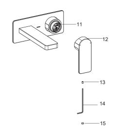
Turn off the valve, and loosen the screw(13) in the handle (12) with hex wrench(14). Install the handle onto the valve base(11) and keep it downward.
