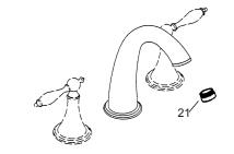
Remove the aerator(21). Open both hot and cold valves and run water through the spout to remove any debris. Turn off the valves. Reinstall the aerator.
