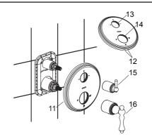
Slide the faceplate(11) onto the valve with slots(12) downwards. **NOTE:** Don't squeeze out the rings(13,14). Push it against the wall.
