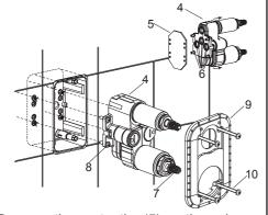
Remove the protection(5) on the valve kit(4). **NOTE:** Don't drop the o-rings(6), don't turn the cartridge spindle(7) when reinstall it. The holes on the bottom in the valve kit should be aligned with the holes in the mounting box. Install the valve kit into the mounting box kit, tighten the screw(8).
