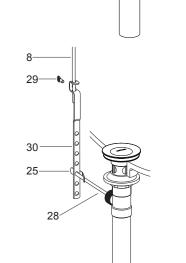
Assemble thumb screw(29) to link(30), and link onto ball lever(28) with 'V'-clip(25). Slide lift rod(8) into the hole in link. Push the ball lever down into the open position, and adjust the lift rod. Tighten thumb screw.
