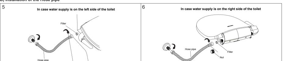
Insert the filter & install the Hose pipe with filter over the threads as shown in figure.Take out the nut. Install the Hose pipe with filter over the threads as shown in figure.Close the opening on the right side with the nut provided.Close the opening on the left side with the nut provided.
