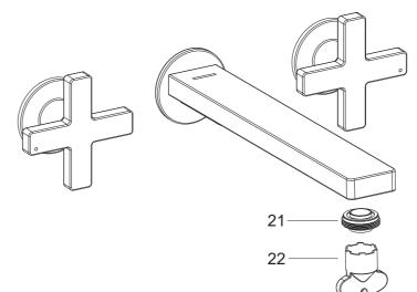
Ensure that all connections are tight. Ensure that the handles are in the off position.
